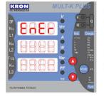
**Energy Measurements:** checking of **kWh+, kWh-, kVArh+, kVArh-, kW** and **kVA** values. To access this mode, hold
